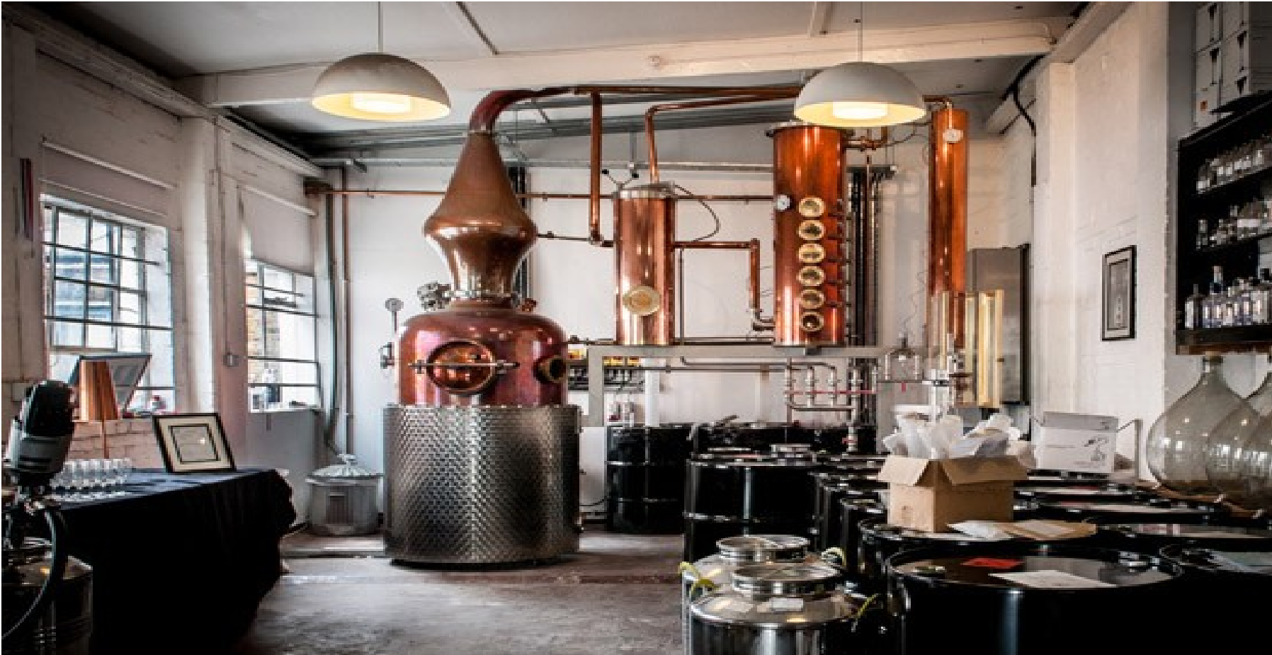
Picture 1: Modern small vodka distillation column
