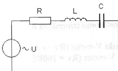
$$R = 20\Omega, L = 50\text{mH}, C = 47\mu\text{F}, U = 230\text{V}, f = 50\text{Hz}$$
