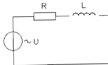
$$R = 20\Omega, L = 0,1\text{ H}, U = 230\text{ V}, f = 50\text{ Hz}$$
