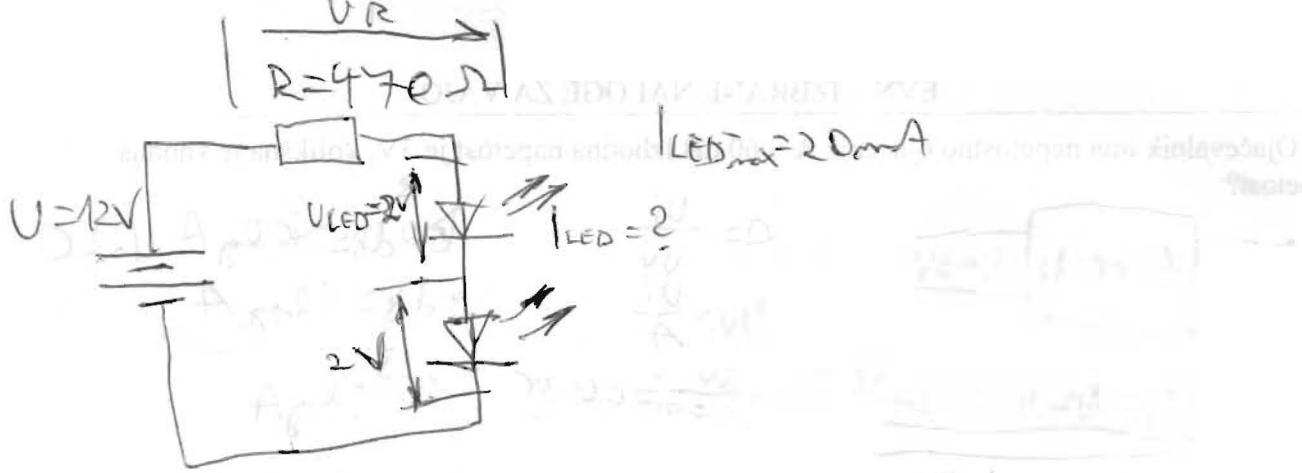
$$I_{LED} = \frac{V_R}{R} = \frac{V - 2V_{LED}}{R} = \frac{8V}{470\Omega} = 17mA$$
