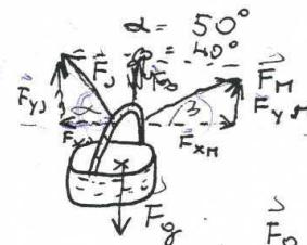
$$\begin{aligned} F_M &\approx F_{yM} \\ \cos \alpha &= \frac{F_{yM}}{F_M} \\ \sin \alpha &= \frac{F_{xM}}{F_M} \end{aligned}$$
