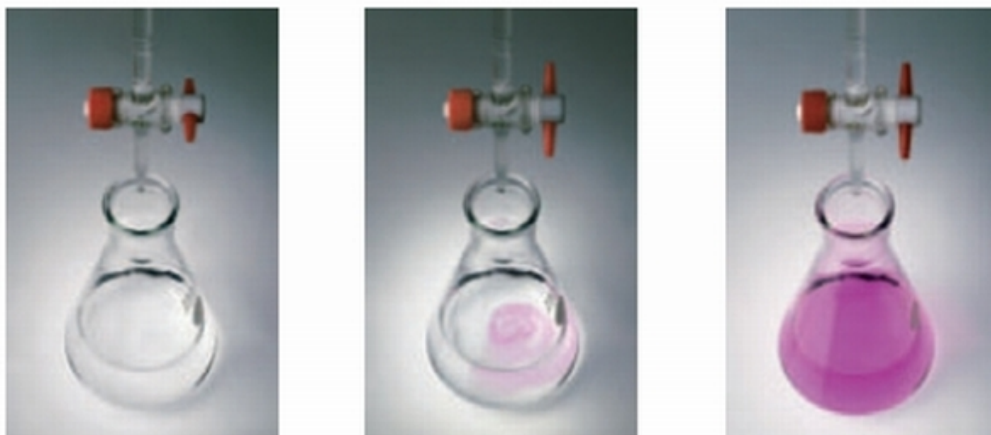
▲ FIGURE 4.18 Titration In this titration, NaOH is added to a dilute HCl solution. When the NaOH and HCl reach stoichiometric proportions (the equivalence point), the phenolphthalein indicator changes color to pink.
